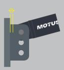
Double check clearance between ram and mounting plates
